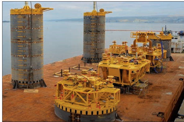
Kizomba Satellites Phase 2 subsea equipment was installed in 2,200 to 4,000 feet of water.
