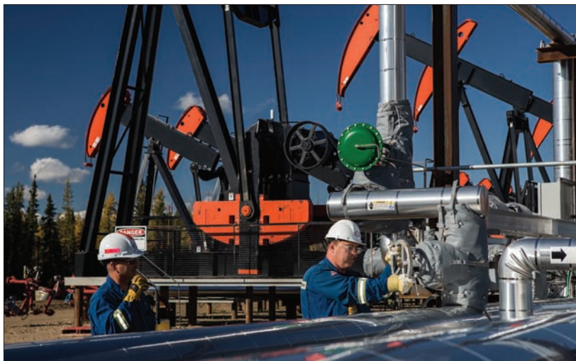
At the Cold Lake heavy oil field in Alberta, bitumen is extracted by injecting steam into the ground.
