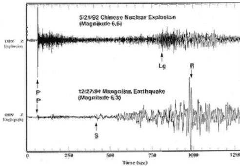
Example from a 1992 nuclear test at the Lop Nur test site in China, as recorded in Russia. Ground motion compared to an earthquake that occurred nearby. Both seismic signals have traveled a similar distance and should show similar amounts of attenuation.
