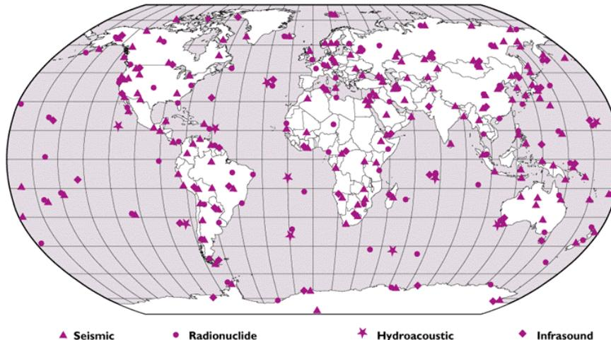
Worldwide, the International Monitoring System will consist of 321 monitoring facilities to help detect possible violations to the comprehensive nuclear test ban treaty. Approximately one-third of the planned monitoring stations are currently operational.
