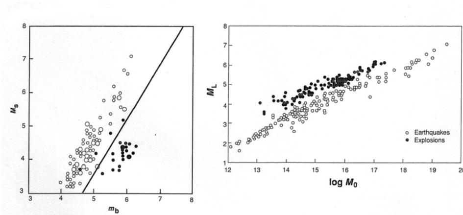
Left :Fowler 4.11a. Earthquakes and explosions in Eurasia. Solid line shows bounds between earthquakes and explosions.  $m_b = 2.87 + 0.6M_S$
